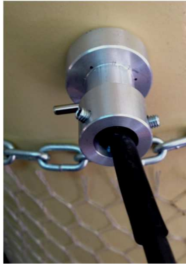
Hydrogen flow through the steel wall of a gas cylinder
