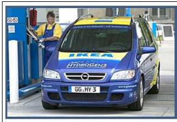
Figure 3: LH 2 – PEMFC system (GM HydroGen 3 FCV)
