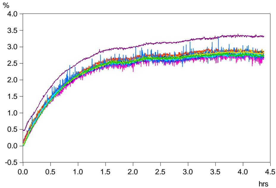
Figure 7 shows a typical set of traces recording H<sub>2</sub> concentration as a function of time, with the hydrogen concentration settling to a steady value. One trace clearly has an offset and was omitted from the subsequent analysis.
