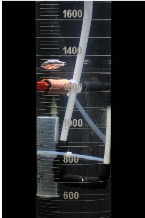
Figure 2: A hydrogen bubble after it has left the open end of a 20 ml syringe.
