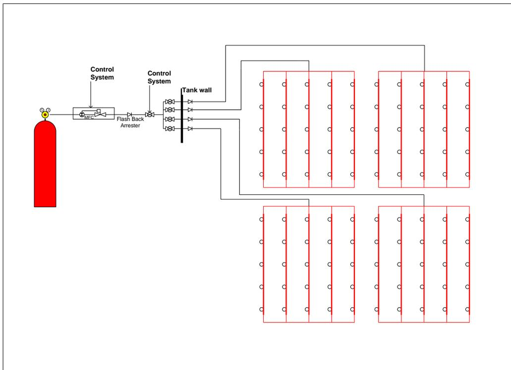
Figure 3: A schematic view of the hydrogen supply and the bubbler array.
