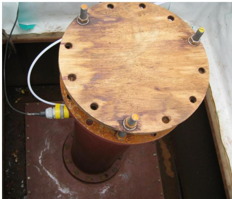
Figure 5: A 300 mm diameter chimney, fitted with hydrogen sensor, manometer tube, wooden cap and showing the bottom of the surrounding shelters
