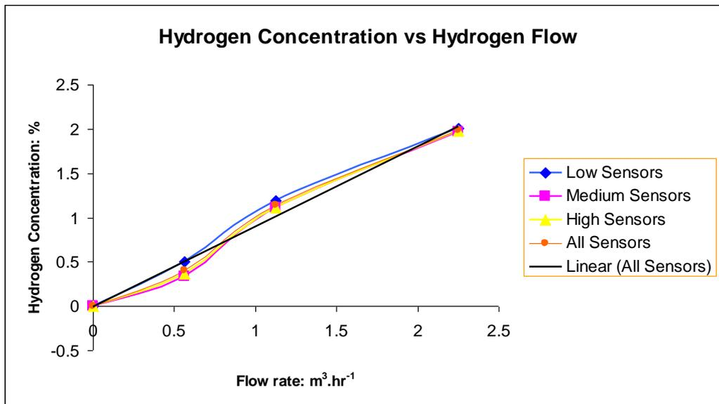
Figure 8: Mean hydrogen concentrations vs. hydrogen flow for 300 mm diameter chimneys located diagonally on the roof, separated by approximately 6.3m., with hydrogen flow bubbling over all quadrants. As would be expected, the hydrogen concentration is proportional to the flow rate.
