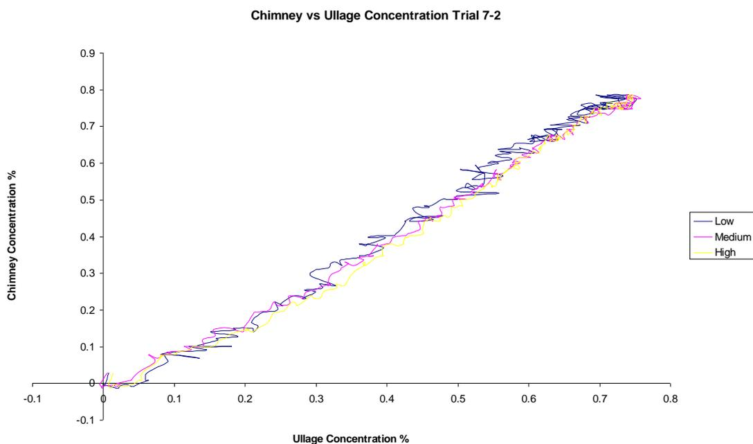
Figure 9: Chimney hydrogen concentrations vs. mean hydrogen concentrations for 300 mm diameter chimneys located diagonally on the roof, separated by approximately 6.3m., with hydrogen flow bubbling over all quadrants.
