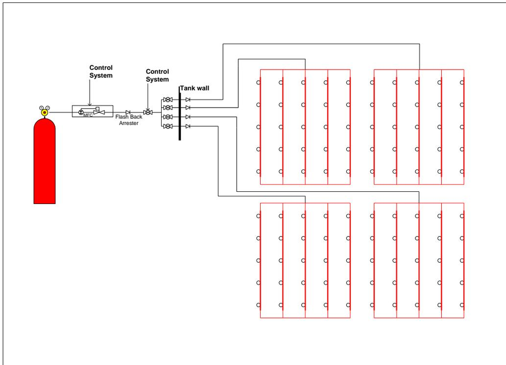
Figure 3: A schematic view of the hydrogen supply and the bubbler array.
