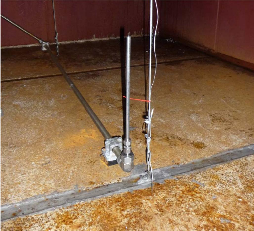
Figure 3. Photo of the hydrogen release point within the enclosure
