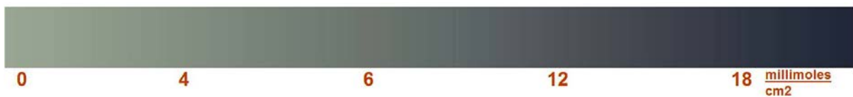
Figure 1- Color calibration of MoO_3 based “smart paint” as a function of hydrogen exposure.
