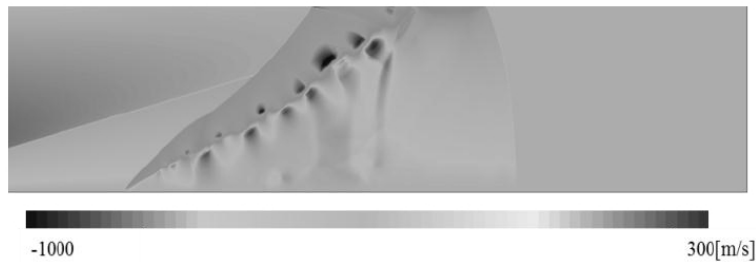
Fig. 5 y -direction velocity profiles for burst pressure of 14.6 MPa at 14.0 ms.
