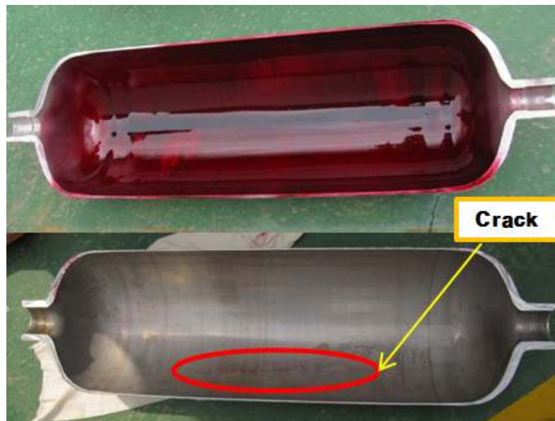
Figure 4. Penetration Test for Inner Liner of Type-3 Cylinder
