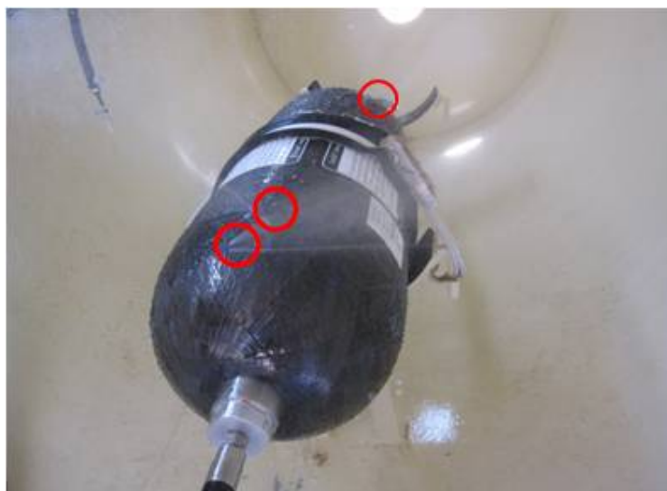
Figure 3. Leakage of Type -3 Cylinder
