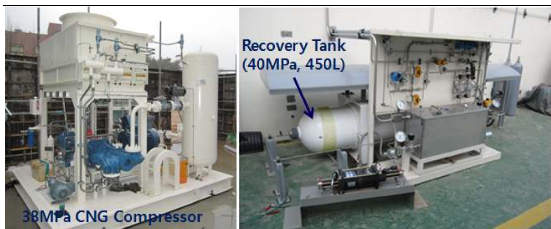
(b) Compressing and Recovery Equipment for Natural Gas(Max pressure: 38 MPa)
