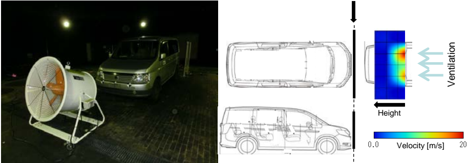
(a) Blower 2 m forward to vehicle; wind velocity distribution on vehicle front
