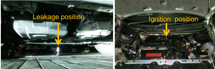
Figure 19. Leakage from engine compartment base center and ignition at firewall top center
