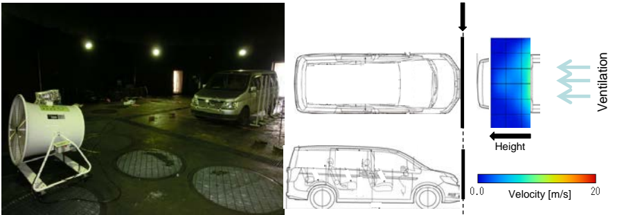
(b) Blower 5 m forward to vehicle; wind velocity distribution on vehicle front
