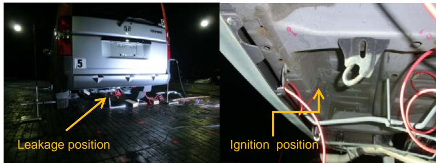
Figure 17. Leakage from rear-floor center and ignition on reverse side of rear bumper
