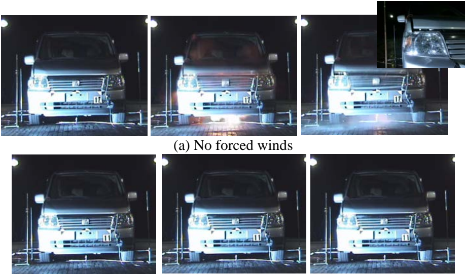
(a) No forced winds (b) Winds from 5m forward to vehicle Figure 21. Sequence photographs of ignition
