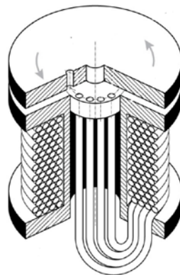
Figure 1. Schematic view of capillary vessel for hydrogen storage
