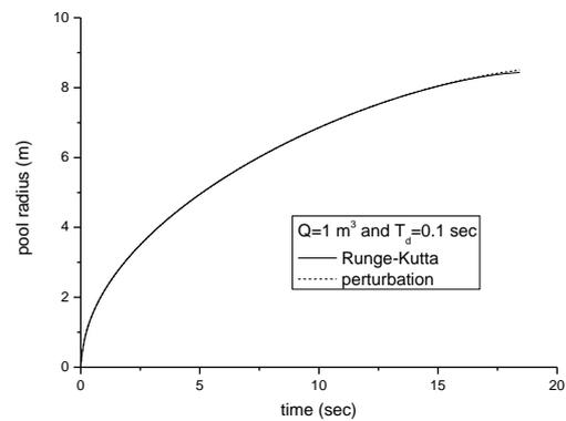
Figure 4. Pool radius vs. time with  $T_d=0.1$  s.
