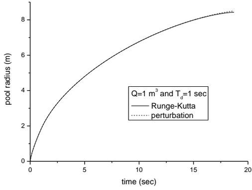
Figure 5. Pool radius vs. time with  $T_d=1$  s.
