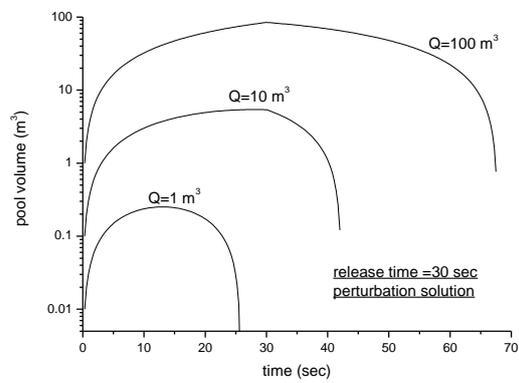
Figure 8. Pool spread pattern with spill volume
