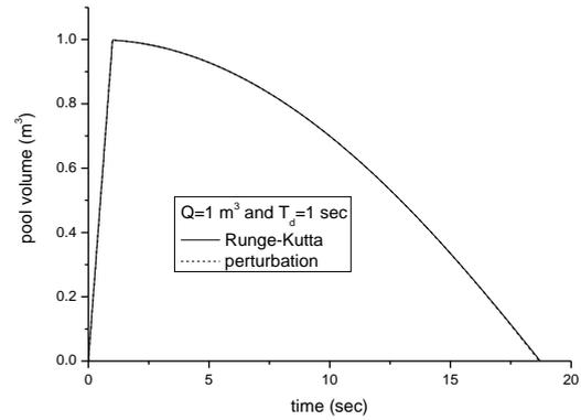
Figure 2. Pool volume vs. time with  $T_d=1$  s.
