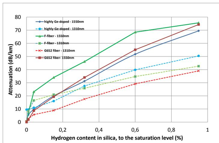
Figure 4: Measured attenuations at 1310nm and 1550nm for the three fibres, as a function of hydrogen content in silica
