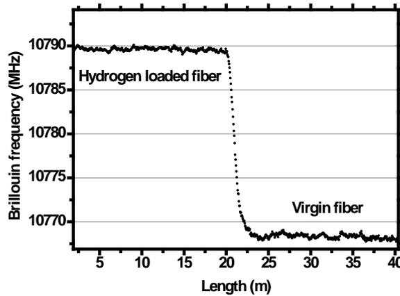
Figure 5: Measured maximal Brillouin frequency as a function of the distance along an optical fiber line made of hydrogenated and saturated sample and virgin (dummy) coils.
