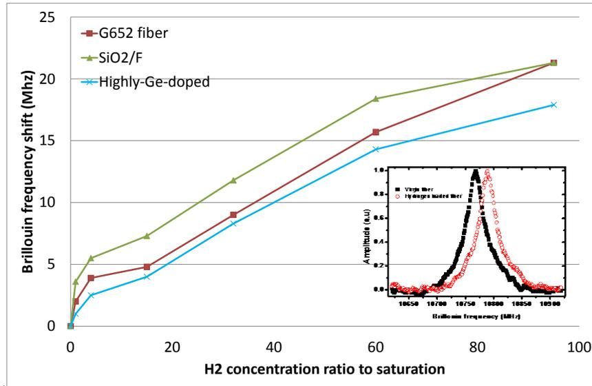
Figure 6: Measured Brillouin frequency shifts in 3 optical fibers as a function of calculated hydrogen content ratio to the saturation level in the silica core.
