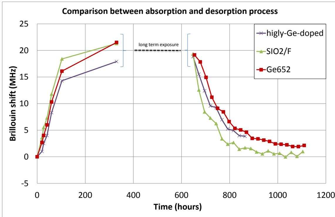
Figure 7: Brillouin frequency Shift during the sorption and desorption period
