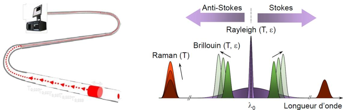
Figure 1: Backscattering spectrum of a monochromatic wave within an optical fiber.
