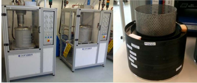
*Figure 2: Picture of the pressurized chambers and coil sample*
