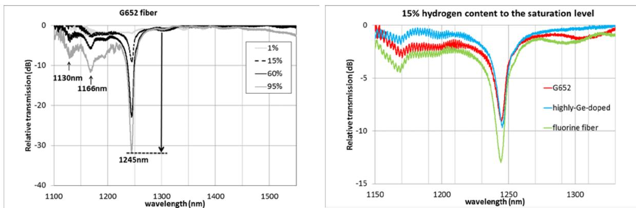
Figure 3: (left) Measured spectral transmission for three hydrogen contents, in the G652 fiber and (right) Focus on the 1245nm absorption peak, after 41h exposure to hydrogen, for the three fibers
