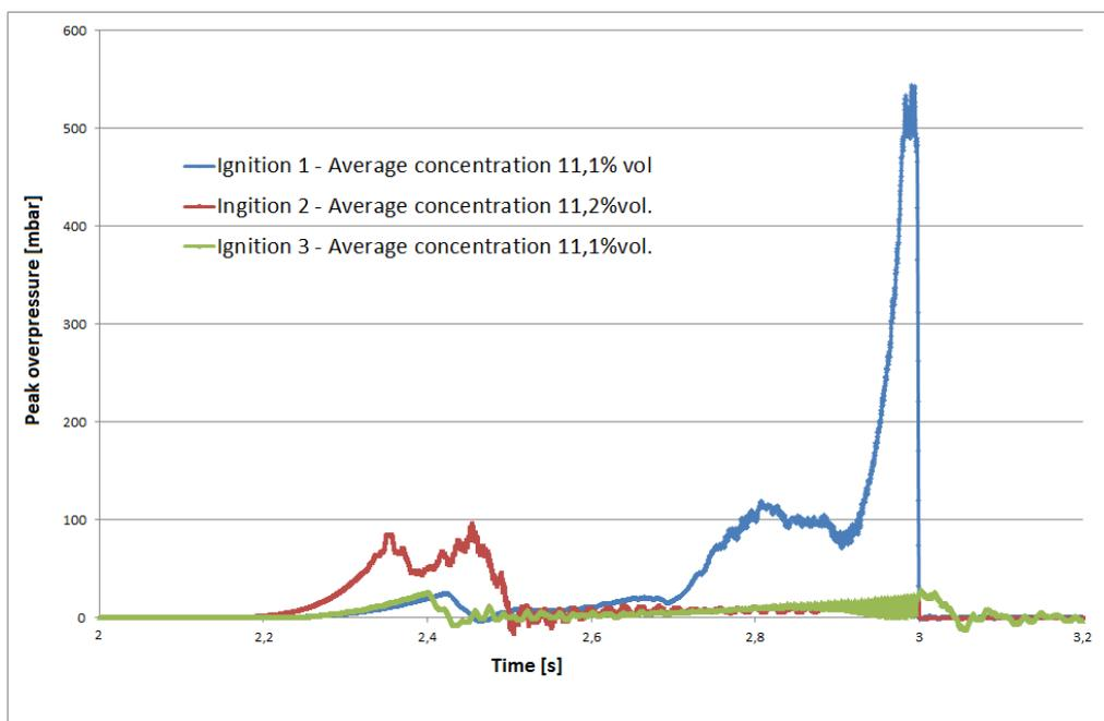
Figure 9 – Effect of ignition location on RED-CVE internal pressure vs. time history for 11,1% H<sub>2</sub> concentration and RED-CVE vent dimensions 0,205 mm X 0,205 mm
