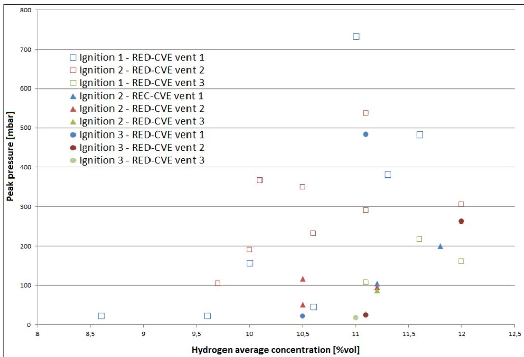
Figure 7 – Maximum peak overpressure inside the RED-CVE vs. H<sub>2</sub> average concentration for different ignition location and RED-CVE vent dimensions
