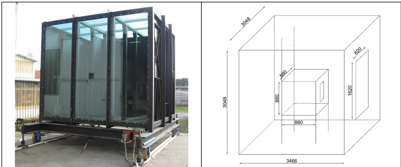
Figure 1 – Photo of the CVE test facility (left) and its dimensions [mm] (right)
