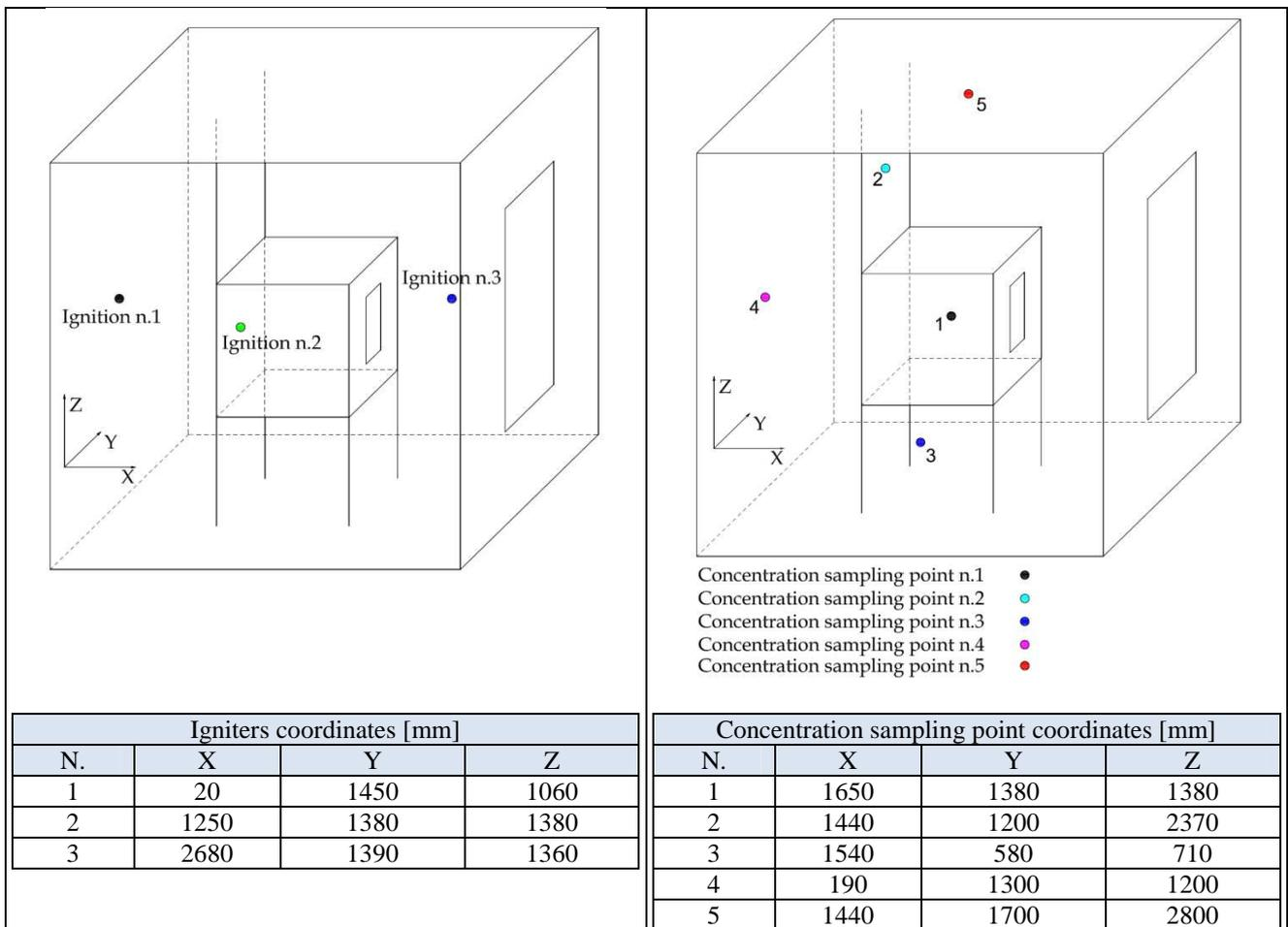
Figure 3 – Igniters position and coordinates (left) and concentration sampling points position and coordinates (right)
