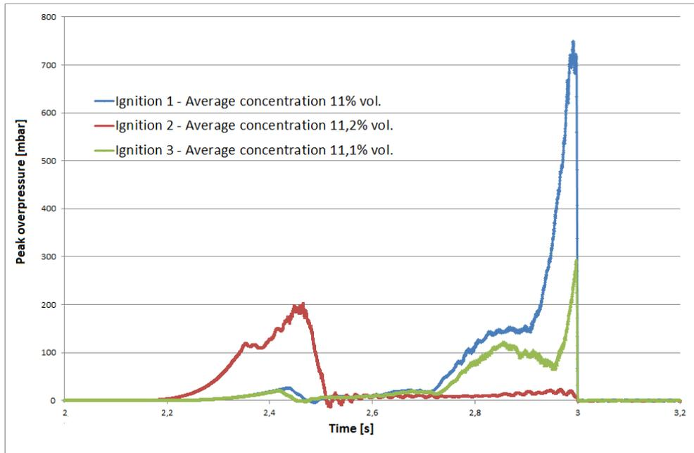
Figure 10 – Effect of ignition location on RED-CVE internal pressure vs. time history for 11,1% H<sub>2</sub> concentration and RED-CVE vent dimensions 0,135 mm X 0,205 mm
