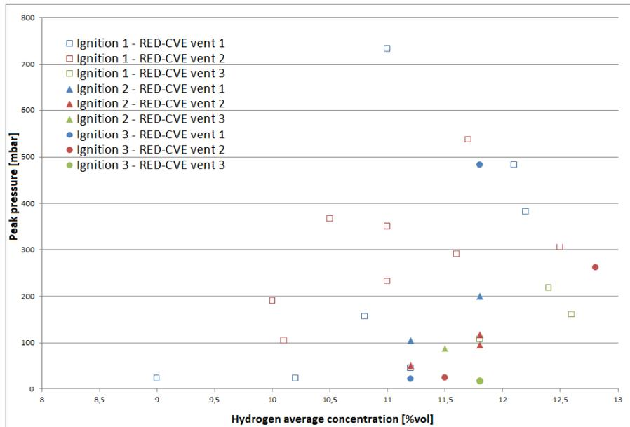
Figure 8 – Maximum peak overpressure inside the RED-CVE vs. H<sub>2</sub> concentration measured inside it for different ignition location and RED-CVE vent dimensions
